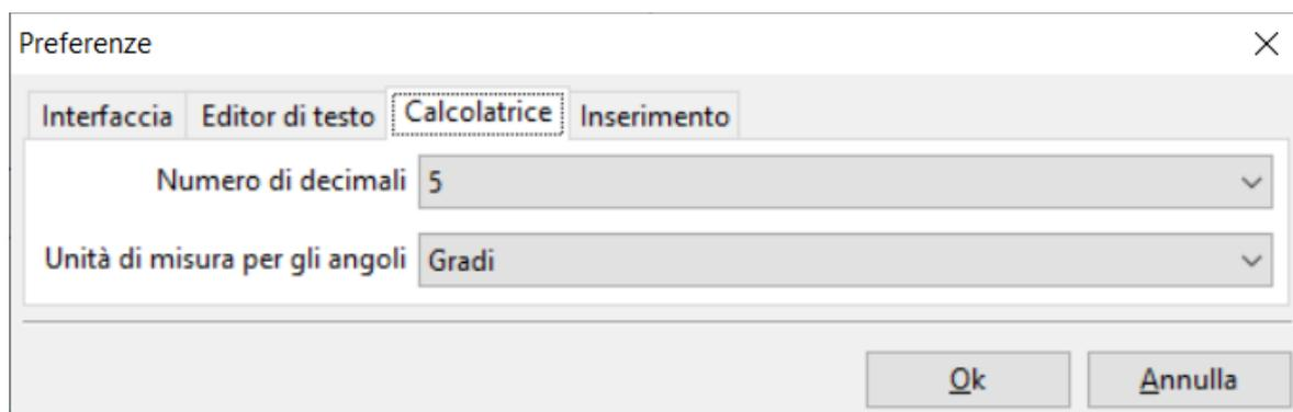
For the "calculator" tab, there are two choices: Number of decimals for the calculator (value from zero to five) Unit of measure for angles with three choices: degrees, radians, or gradients
